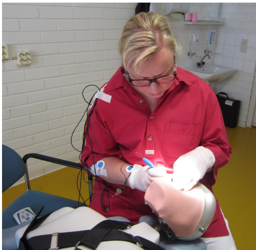
Figure 2. The simulated work situation using plastic model teeth attached to a phantom head fixed to a dental chair. Here are two test subjects working in their own simulations.
