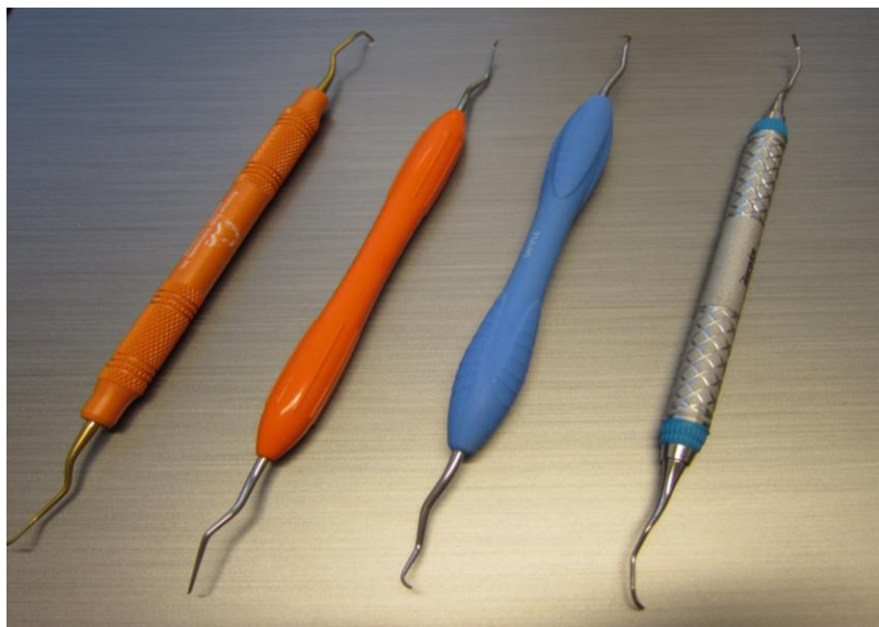
Figure 2. The tested four instruments, from left to right: A, American Eagle Instruments, Inc. Gracey curette AE G 11-12 XPX B, LM 211-212M XSI, GRA 11-12 (LM ErgoMax) C, LM prototype D, Hu-Friedy SG11/129
